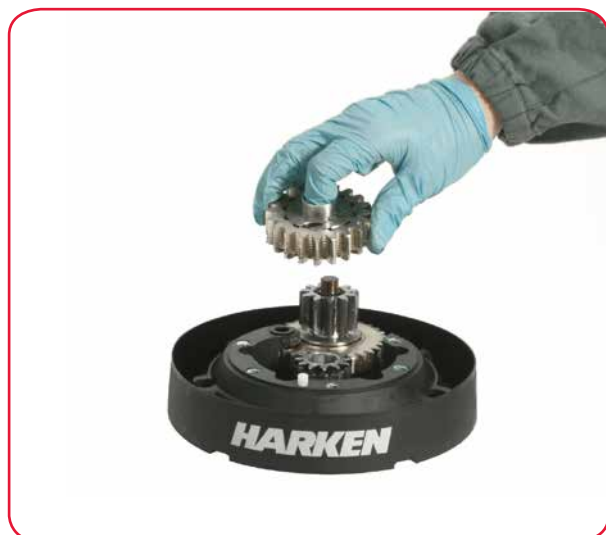
7. Remove the gear and remove the pawls carrier.
